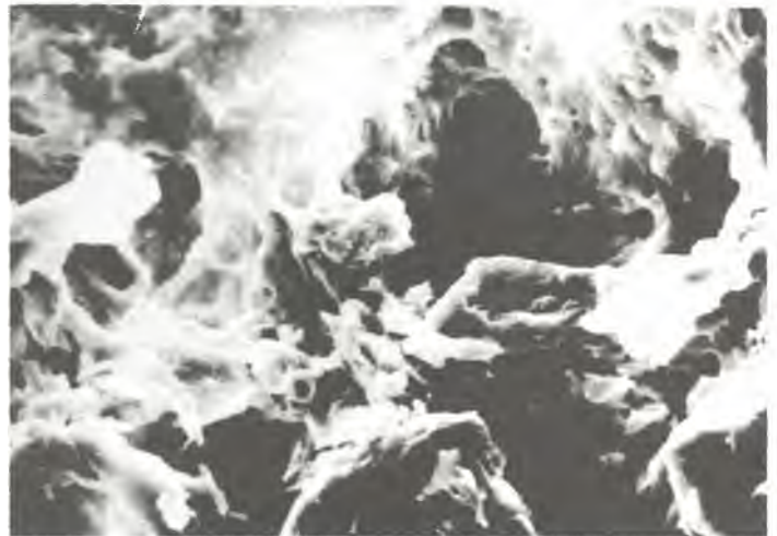
FIGURE 3 SCANNING ELECTRON MICROGRAPH AFTER 2 MONTHS SOIL BURIAL (1000X)
