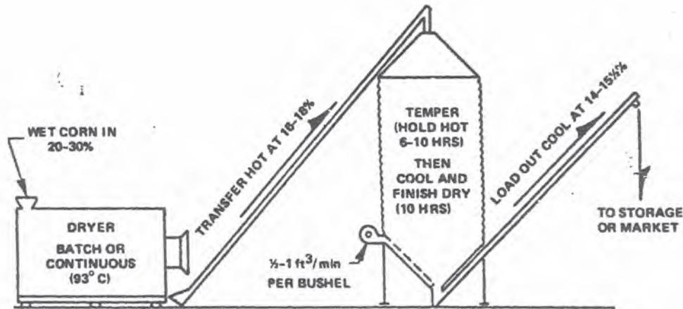
FIGURE 14.—Schematic flow diagram of drying process. (Courtesy of Coop. Ext. Serv., Purdue Univ.)
