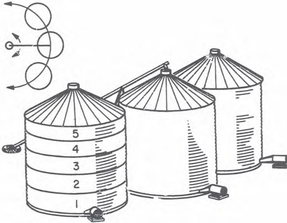
**FIGURE 9.**—In-bin layer drying with supplemental heat. Bins are filled in rotation, one layer at a time. As each layer partially dries, successive layers are added until storage is full and the grain is dried in place. (Courtesy of Bruce McKenzie, Purdue Univ.)
