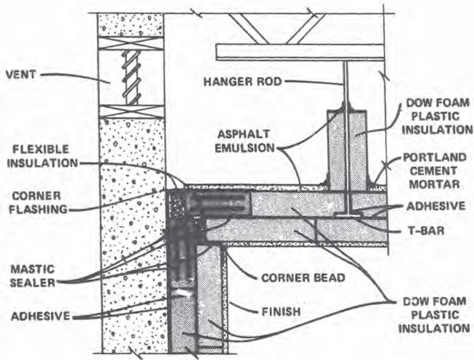
FIGURE 30.—Construction utilizing suspended T-bar ceiling and foam plastic insulation for seed storage facility. (Courtesy of Amspec, Inc.)
