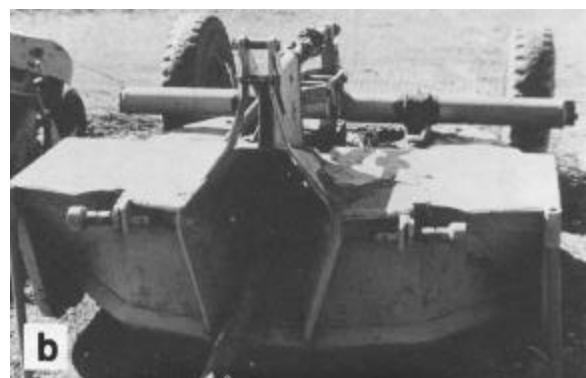
Figure 16. (a) MEDC reciprocating root pruner and (b) tractor-drawn rotary mower used for top mowing both control seedling growth.
