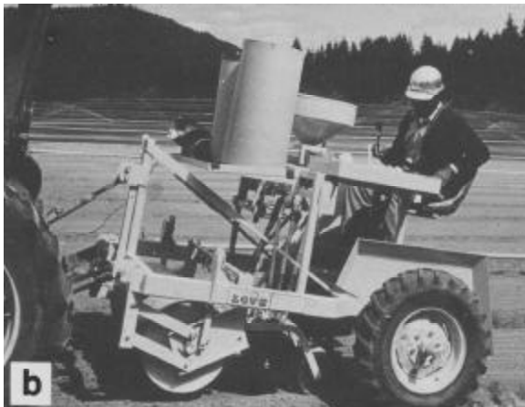
Figure 9. Drill seeders like the (a) Wind River and (b) Love-Øyjörd are commonly used to sow nursery seed.
