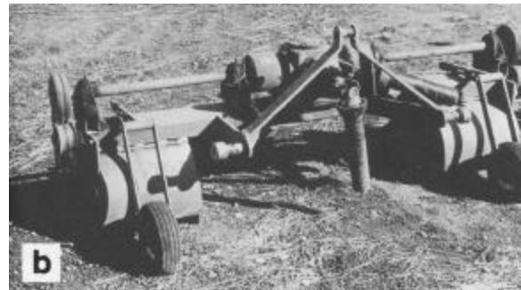
Figure 15. (a) Budding wheel hoe row cultivator and (b) Coeur d'Alene path cultivator keep nursery beds weed free.
