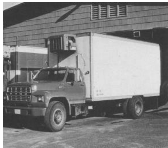
Figure 24. Seedlings are often transported to the field for outplanting in refrigerated trucks.
