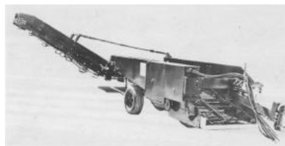
Figure 20. Grayco Harvester, which lifts seedlings mechanically rather than manually.
