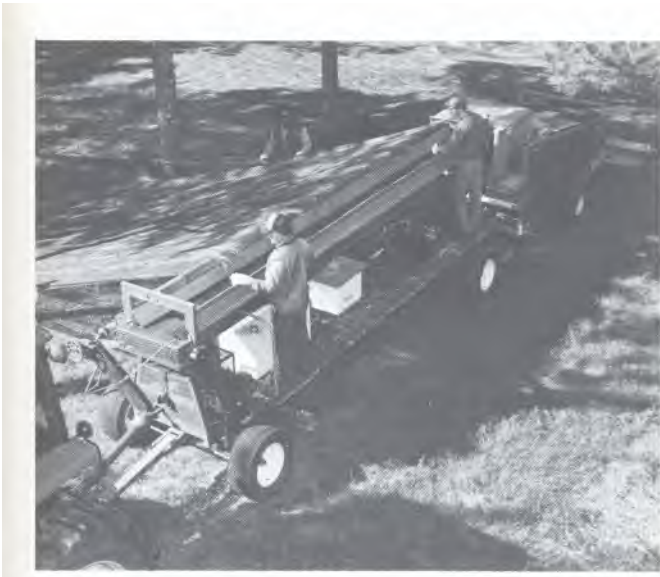
Figure 4.3. Net retrieval system equipment developed by the U.S.D.A. Forest Service for collection in southern pine seed orchards.
