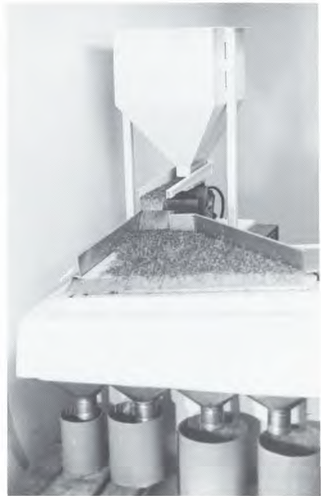
Figure 4.8. Two machines commonly used to condition seeds of southern pine: (A) aspirator; (B) gravity table.
