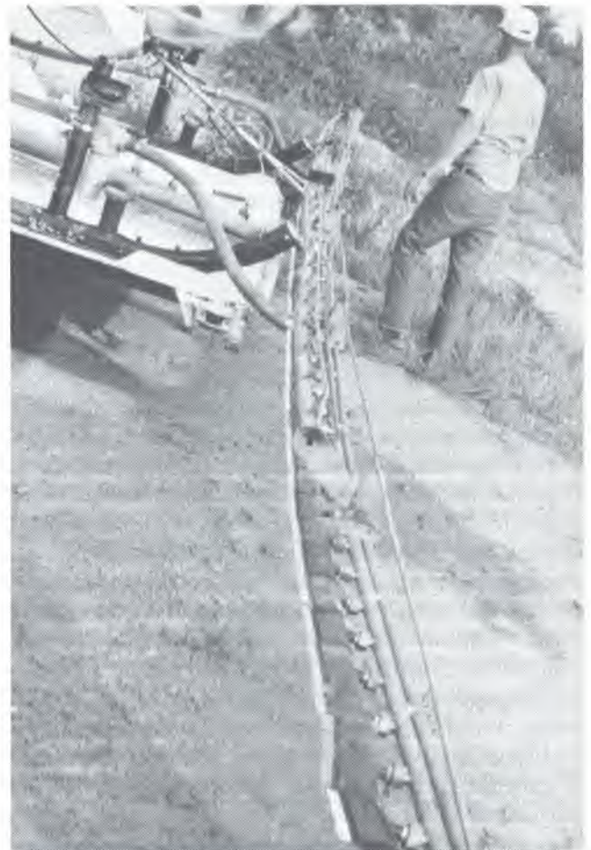
Figure 19.6. The Microfoil® boom, commonly used for aerial herbicide applications, is designed to minimize fine spray droplets, which are prone to drift.
