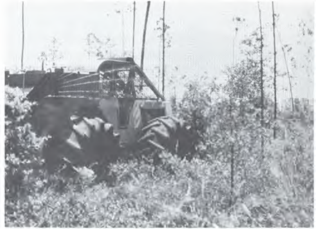
Figure 19.9. Ground sprayer equipped with a manifold nozzle system utilizing straight-stream nozzles to apply solutions of soil-active forestry herbicides.
