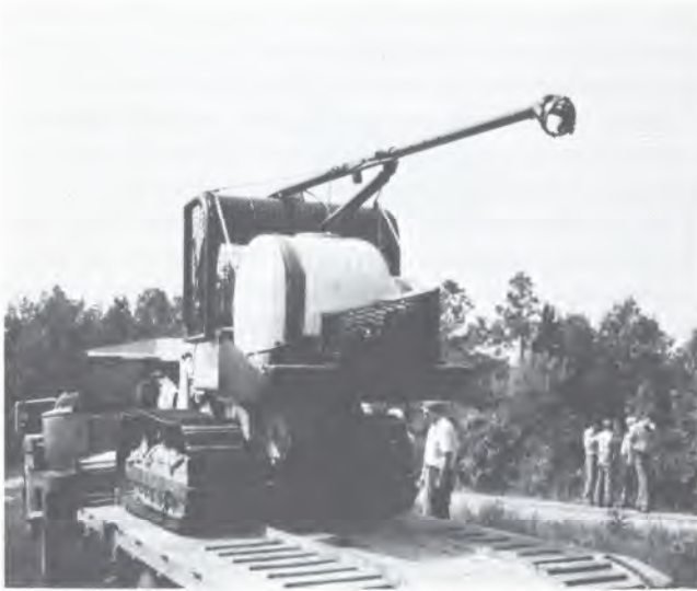
Figure 19.8. Tractor-mounted ground sprayer equipped with a cluster nozzle, which is raised or lowered to obtain adequate coverage of treated vegetation.
