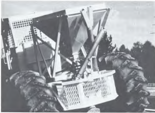
Figure 19.7. The Omni® spreader, used to apply solid herbicide formulations, provides uniform herbicide distribution across a 28-m effective swath.
