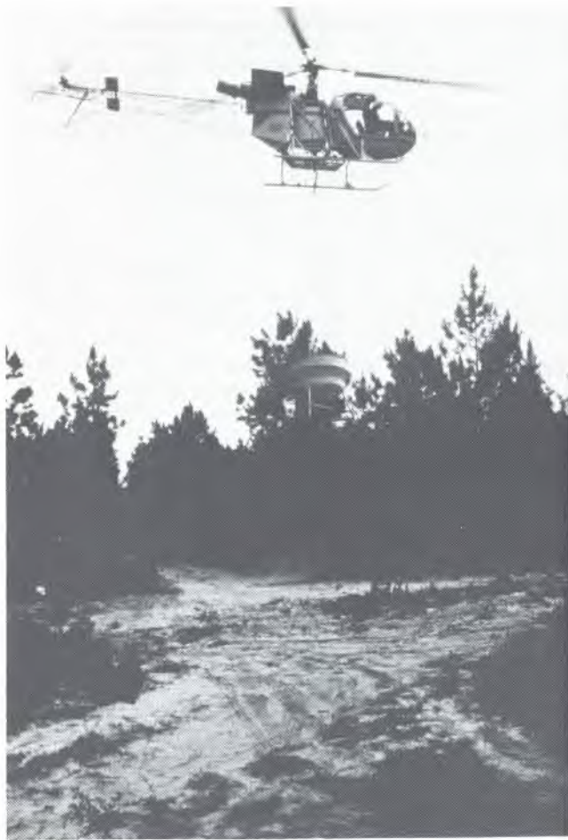
Figure 19.5. Modified fertilizer spreaders are commonly used to apply solid formulations of forestry herbicides.
