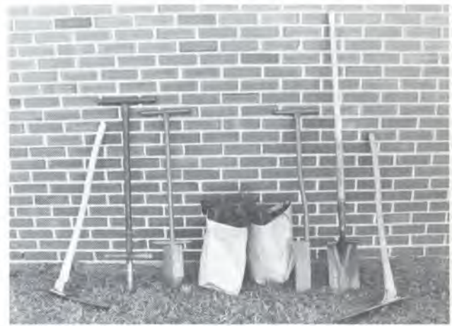
Figure 17.4. Hand tools commonly used for planting in the South: (from left to right) hoedad with concave blade and regular bracket, cylindrical dibble for container seedlings, KBC dibble bar, double planting bag with belt, OST dibble bar, long-handled planting shovel, and hoedad with flat blade and Earp bracket. (Tools provided for photograph courtesy of Forestry Suppliers Inc.)
