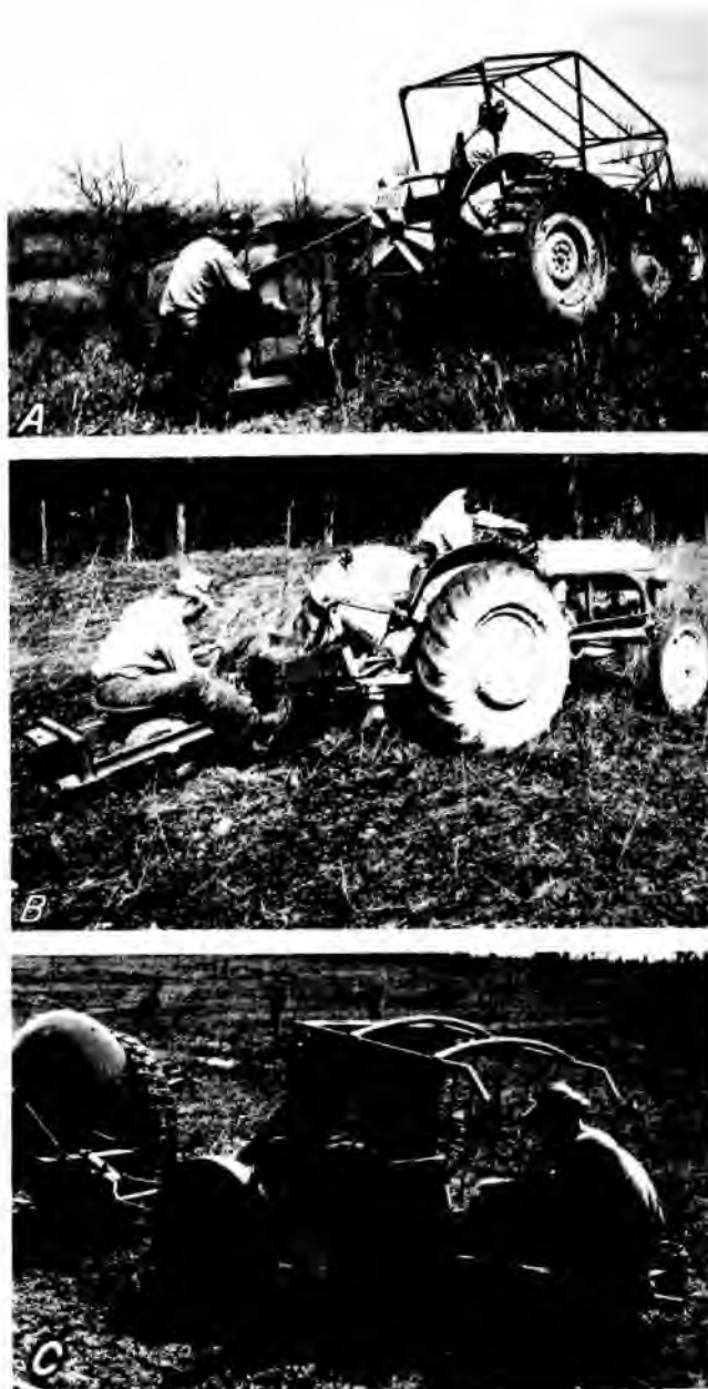
Figure 26.—Three types of tree-planting machines in common use: A, Floating type; B, semifloating type; and C, the trailer type (photo courtesy of Ohio Power Co.).
