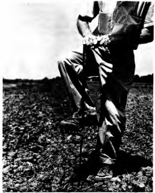
Figure 28.—Planting rods, from \frac{1}{2} - to \frac{3}{4} -inch iron, can be easily made by your local blacksmith. For planting poplar cuttings.
