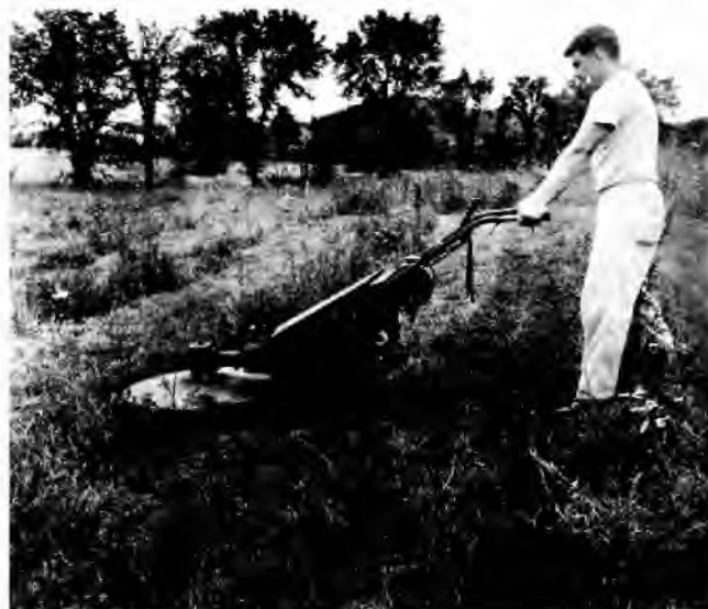
Figure 29.—One type of rotary mower used extensively for the control of grass and weed cover in plantations.
