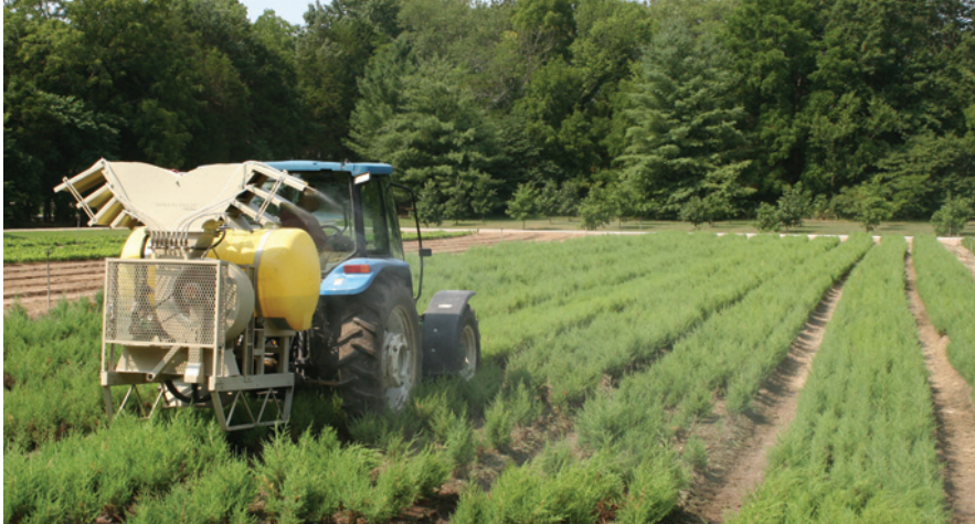
Figure 1.5 —This modified orchard sprayer applies pesticides thoroughly to seedlings being grown at the Missouri Department of Conservation George O. White Nursery at Licking. Photo by R. Kasten Dumroese, USDA Forest Service.
