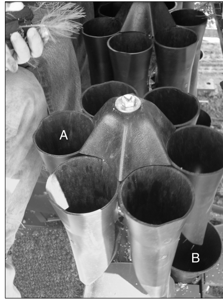
Figure 2. Carousel transplanter – Q-plug is placed in chamber (A) which rotates the plug 180 degrees and drops it into tube (B) which delivers it to the soil.
