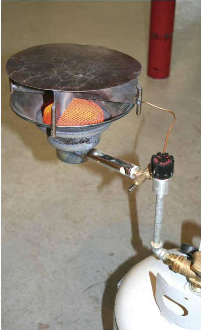
Figure 1. Hot plate mounted on a propane heater used for conducting “pop” tests at the Aberdeen Plant Materials Center.
