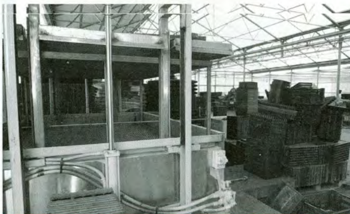
Small, thin-walled trays are cleaned in this cooker for 10 minutes at 170 degrees.
