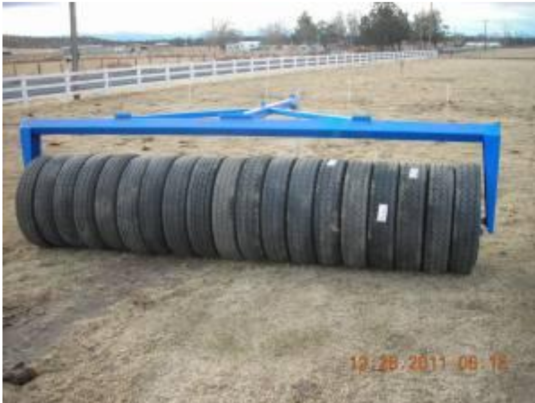
Figure 4. Rubber tire roller packer. A very effective tool to increase broadcast big sagebrush seed contact with the soil and improve establishment.
