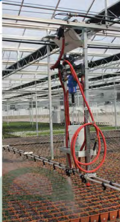
This Cherry Creek Systems Double Rail Boom is using a Dosatron 20gpm injector to apply fungicide to the crop below.
