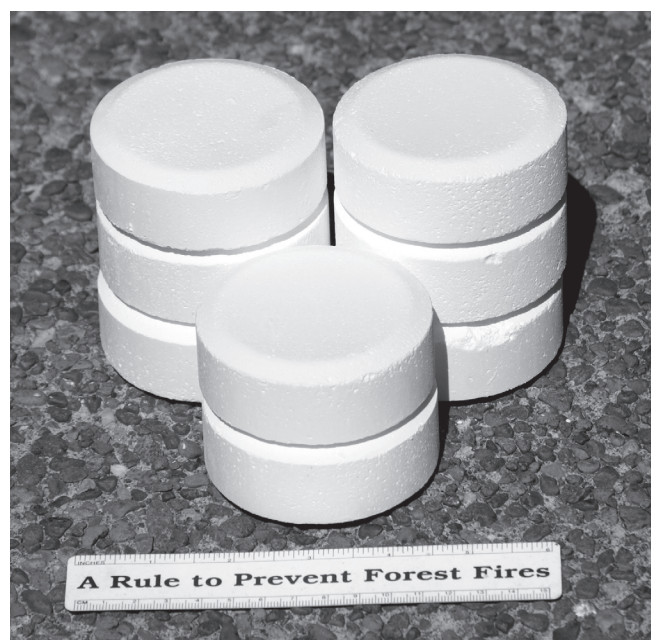
Figure 5 - Tablets are considered the safest way to supply chlorine or bromine for disinfecting irrigation water (Ferraro and Brenner 1998).
