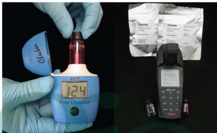
Sanitizing agents can be measured using colorimetric test kits combined with a pocket colorimeter. A reagent is added into the solution, and a digital meter interprets the color change as a concentration. The HI 701 Checker HC Handheld Colorimeter (left) measures free chlorine, and the Thermo Scientific Orion AQUAfast AQ4000 Colorimeter (right) can be programmed to measure virtually all the sanitizing agents. Photos by Jinsheng Huang and Dustin Meador
