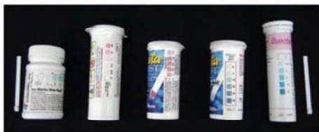
TOP: Monitoring water quantity, quality and drainage is best done preventatively, rather than after problems occur. Photo by Paul Fisher BOTTOM: Sanitizing agents can be monitored using test strips. The test strips above are used to measure (from left to right) free chlorine, chlorine dioxide, copper, peracetic acid and hydrogen peroxide. Photo by Jinsheng Huang
