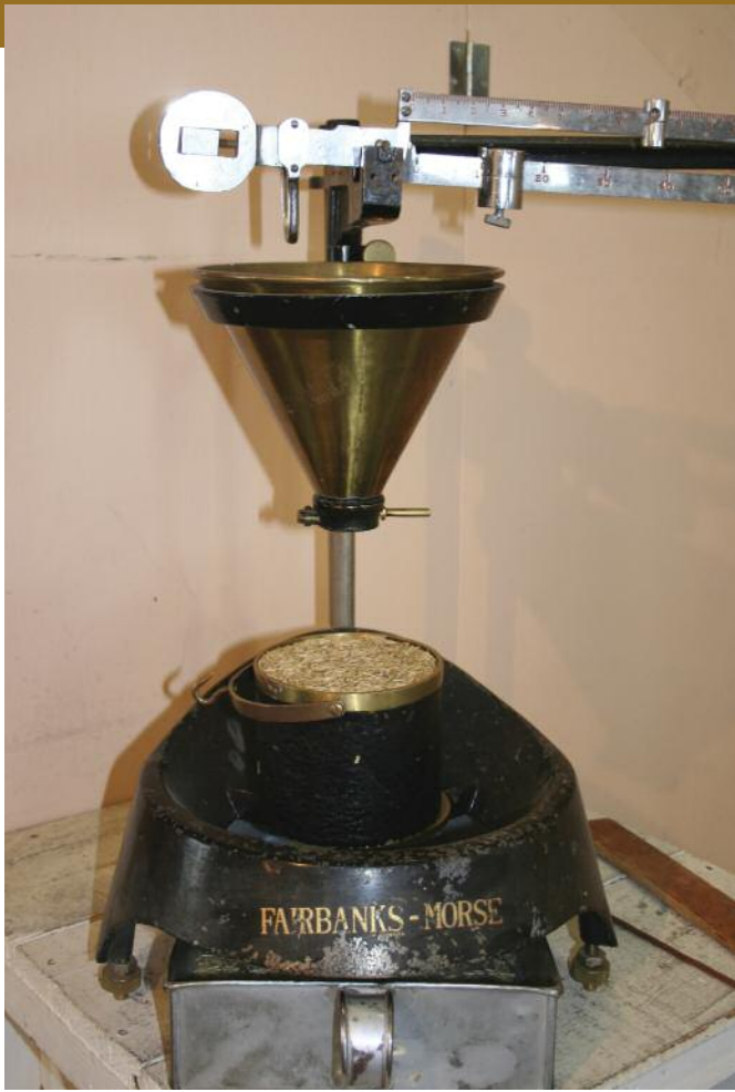
Figure 1. Bushel equivalent scale at the Aberdeen Plant Materials Center. Photo by Derek J Tilley
