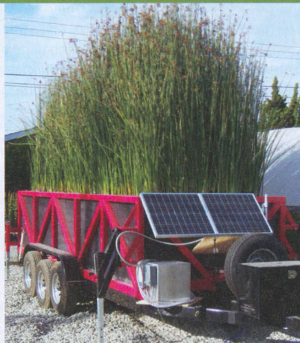
Water moves through this portable subsurface flow constructed wetland, which is established with bulrush, via a solar-powered pump.
