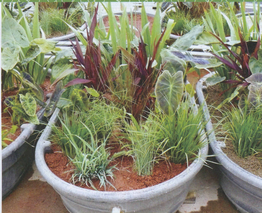
Subsurface flow constructed wetlands lined with fired-clay media and planted with phosphorus hyperaccumulators can consistently remove phosphorus from nutrient-rich runoff.
