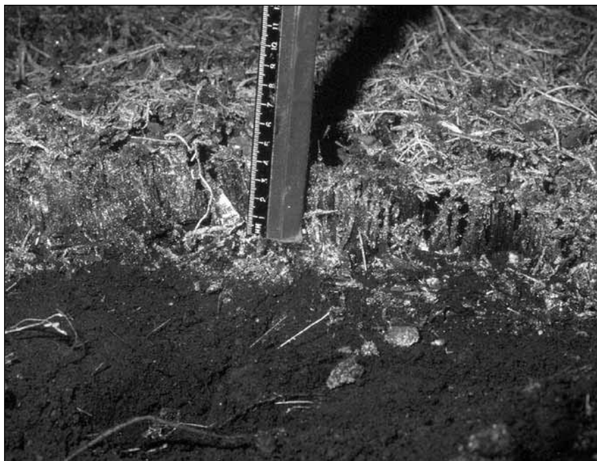
Figure 13. Example of frost action on basalt soil at Unit S-3 (Wing Mountain, AZ) during one night. This is an example of a 'palisade' layer of ice. Careful examination reveals extruded plant material on the surface.
