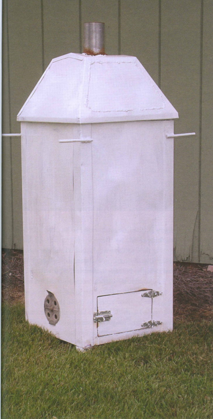
Figure 1. A modified steel trash can makes an ideal combustion chamber for producing smoke to treat seeds.
