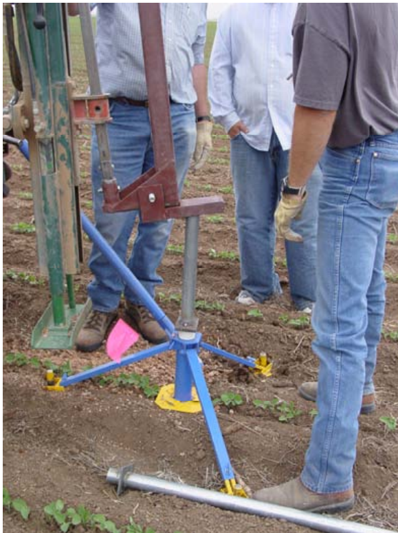
Figure 5.5. Installing access tubes, clockwise from upper left: (1) the Sentek driving head; (2) a steel tube used in conjunction with the hydraulic push machine; the long steel tube prevents the plastic tube from bending. (3) and (4) Using the hydraulic push machine with another steel tube to finish pushing the tube in after the tripod has been removed.
