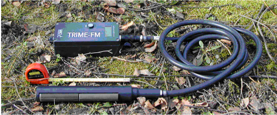
Figure 6.1. The TRIME system from IMKO for profiling soil water content.
