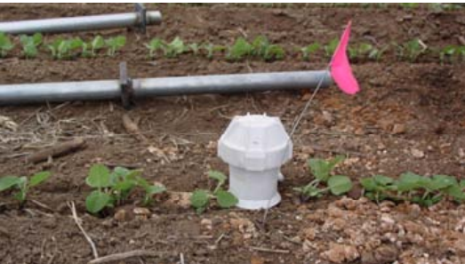
Figure 5.4. Installation of Sentek access tubes, clock-wise from upper left: 1) Tripod adjusted to the vertical, pinned to the ground, and with access tube inserted; 2) Lowering auger into tube from a ladder; 3) Tube nearly installed with horizontal mark that will be at soil surface when finished; 4) Installed tube with top cap; 5) Using a Giddings hydraulic push machine to push the tube 10 cm into the soil
