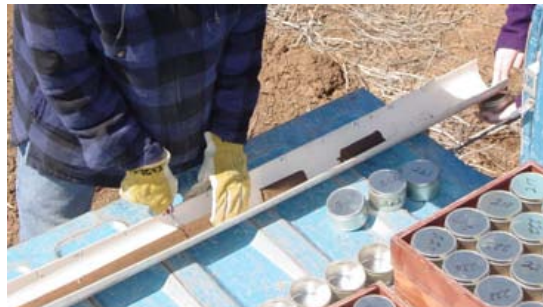
Figure 2.7. (Top left) Example of a “Quick relief” coring tube bit (Giddings Machine Company). To reduce compressive force ahead of the cutting bit, remove the bit material outside of the dotted line. (Top right) A Giddings hydraulic coring machine mounted on a farm tractor being used to obtain a soil core. (Bottom left) Soil core that has been pushed from the coring tube into a semi-circular tray for cutting into samples representative of user chosen depth ranges. The tray is marked at 10 cm intervals. (Bottom right) Once the core has been pushed out of the coring tube, cutting and protection of samples in watertight and vapourtight plastic bags or other containers should proceed as quickly as possible to minimize loss of water to the atmosphere. A 1.5 m core sample can be cut into 10 cm sections and sealed in cans within 3 min.
