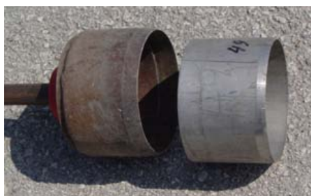
Figure 2.4. (Top) Slide hammer fitted with sampling cylinder. (Left) Close-up of holder for sampling cylinder, showing the internal shoulder against which the cylinder rests during driving. When the cylinder is fully inserted into the soil, the slide hammer is removed and the soil surface is examined for compression by comparing the elevation of the surface inside the cylinder with the surface outside the cylinder.
