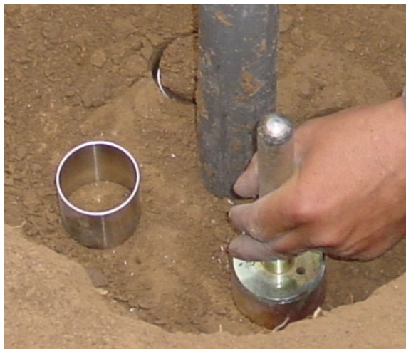
Figure 2.3. (Top) Bevelled volumetric sampling cylinders ( 100 \text{ cm}^3 ), one shown with plastic caps for sample retention (caps may not prevent water loss). (Left) Same cylinders during sampling around the access tube. One cylinder is shown fully driven into soil with no visible compression (top of left photo); another is shown resting on the soil surface prior to sampling; and a third is being driven into the soil with the cylinder holder/driver. (Right) A sampling cylinder made from plastic tubing is shown being driven incorrectly into the soil using a piece of wood as a hammering anvil. This method does not ensure that the force from each blow is transmitted directly down the axis of the cylinder. Off-axis force will cause the cylinder to tip downward on the side where the force is the greatest, causing the soil to shear at the cutting edge as the cylinder rotates.
