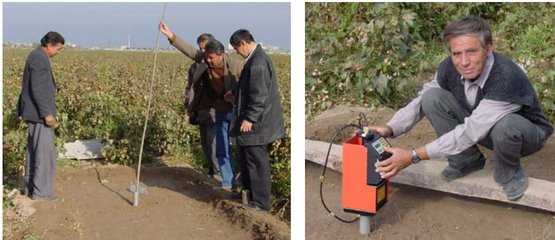
Figure 3.8. (Left) Checking the access tube for water intrusion. (Right) Measurements taken over the entire depth of the access tube will determine the location of the wetting front. Although no depth control stand is shown, one will be used when taking readings for the calibration. (Syrdarya Branch Station, Uzbekistan.)
