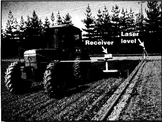
Figure 9—The Spectra Precision Laser Receiver CR600 is mounted to a horizontal arm on the front of the tractor.
