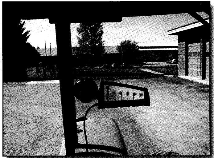
Figure 10—The AGL Precision Laser Receiver MR360R's wireless display mounts inside the cab of the tractor where it is easy for the operator to see.
