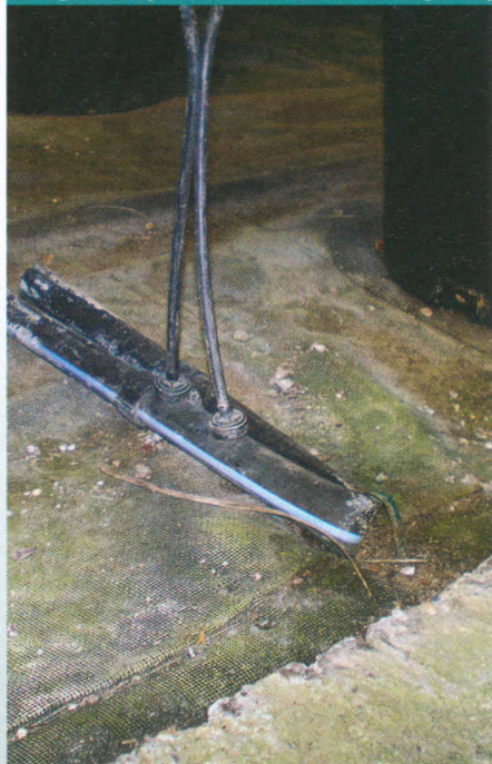
These pressure-compensating emitters deliver a more uniform amount of water to the plants when pressure fluctuates.
