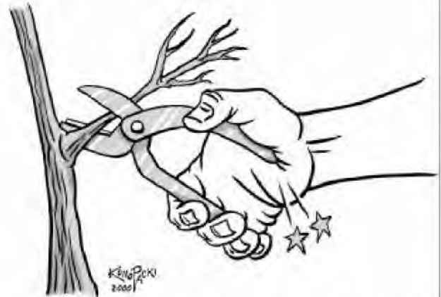
Poorly-designed tool: Handle presses into base of palm and requires user to open after each cut (no spring).
