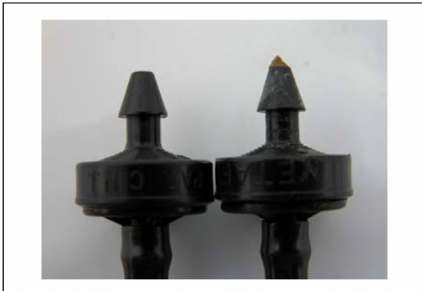
Figure 4. Algae and biofilm cause clogging of drip emitters. New emitter on left, clogged on right.
