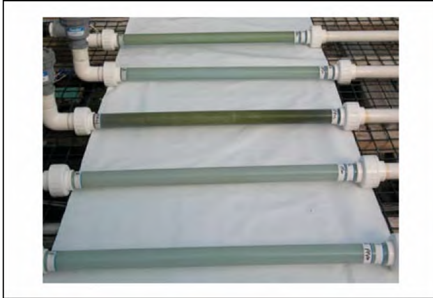
Figure 11. Clear sections of lines following continuous injection of Selectroicide with untreated control in center.
