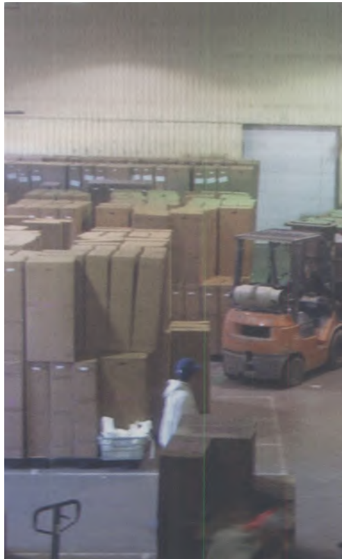
To load a truck in the first bay, the forklift operator travels an extra 22 feet per trip because he has to maneuver around excess inventory that may not be loaded until the end of the day.
