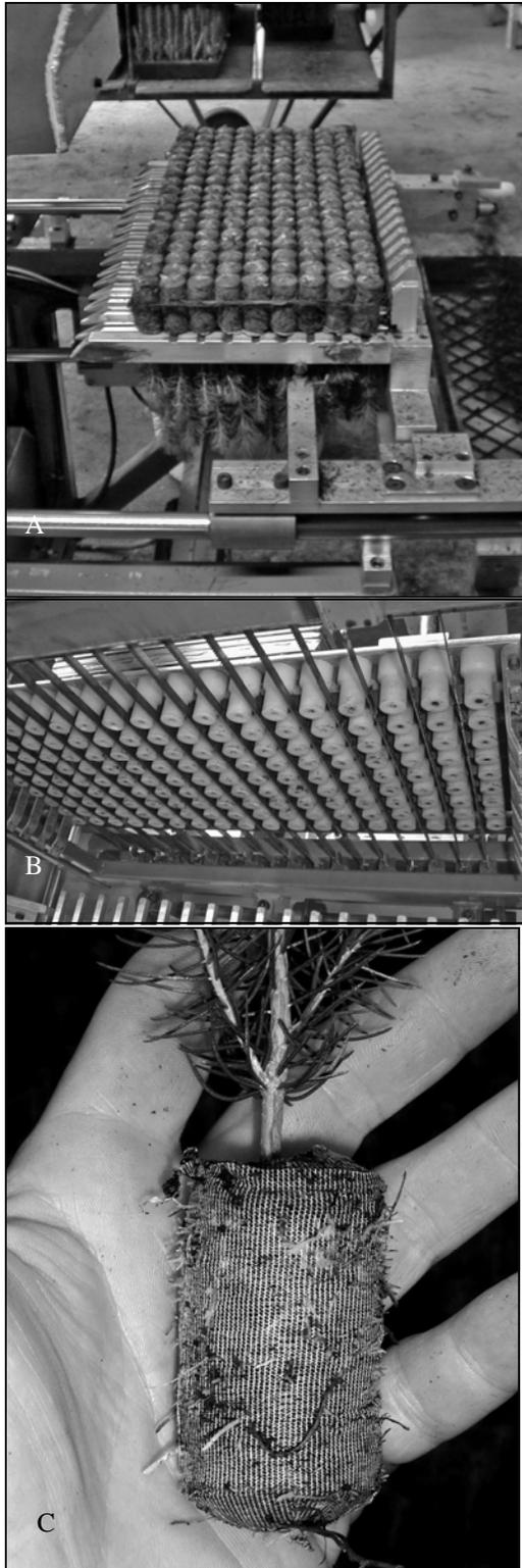
Figure 2 - The Jiffy<sup>®</sup> root pruning machine (A) has thin saw blades that cut root between Jiffy plugs in both directions (B), which produces a box-pruned seedling that is ready for outplanting (C). Photos by Don Willis.
