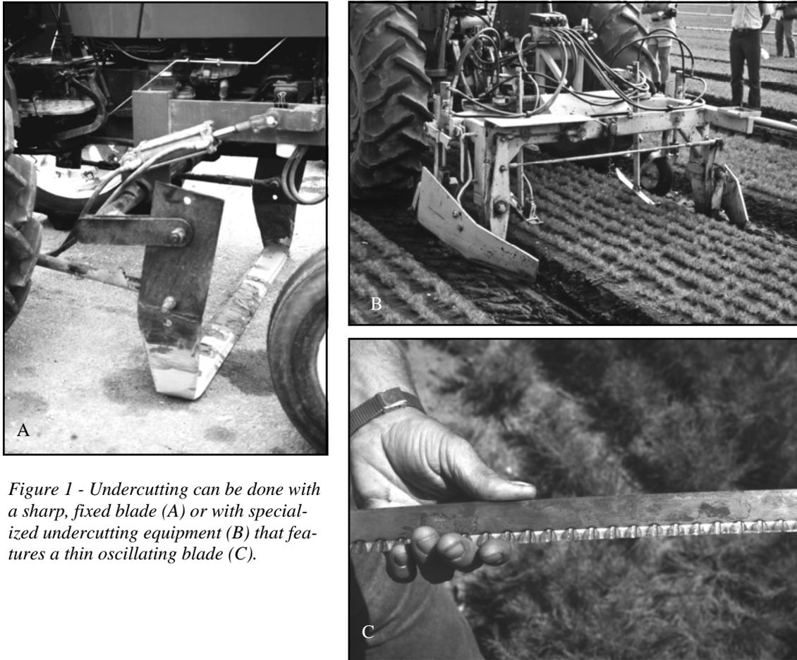
Figure 1 - Undercutting can be done with a sharp, fixed blade (A) or with specialized undercutting equipment (B) that features a thin oscillating blade (C).
