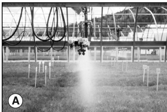
Figure 3 - Cooling the surface of containers is easier with irrigation booms equipped with a mist nozzle (A). Light-colored seed coverings (B) also help reflect solar radiation.
