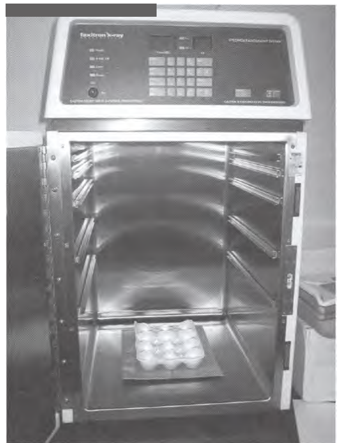
Figure 2 —Indented carton on top of photographic paper on bottom of X-ray machine.
