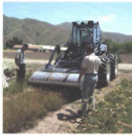
Figure 1. Harvesting wild geranium seeds at Lucky Peak Nursery using the 6 ft wide Woodward Flail-Vac Seed Stripper.
