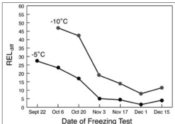
Figure 2. Changes in root electrolyte leakage ( $REL_{diff}$ ) of outdoor grown Norway spruce seedlings measured biweekly from September 22 through December 15.  $REL_{diff}$  is the increased electrolyte leakage from roots following exposure to  $-5^{\circ}\text{C}$  or  $-10^{\circ}\text{C}$  compared with leakage from unfrozen seedlings (Modified from Stattin and others 2000).
