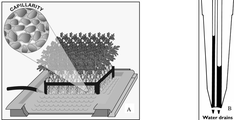
Figure 2 - Subirrigation works because water is drawn upward into the containers by capillarity (A). The amount and speed of water uptake will depend on the porosity of the growing medium, the smaller the pores, the more that will be absorbed (B).
