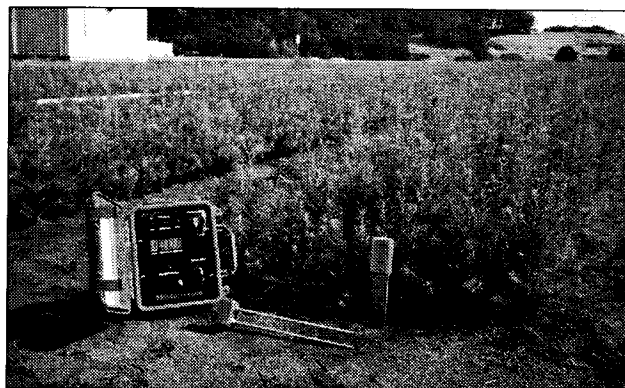
Equip 11A. Moisture-Point TDR™ meters give a digital readout of % moisture using probes that are designed for bareroot nursery soils. (Courtesy of Environmental Sensors, Inc.)
