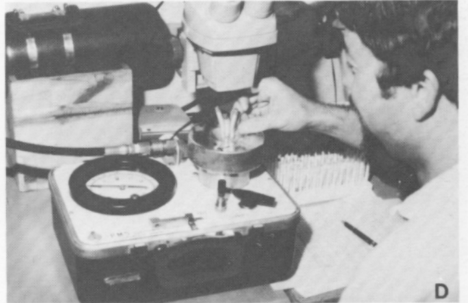
Figure 3. Measuring water status of seedlings: (A) vapor pressure osmometer for the measurement of osmotic potential of plant cell sap, (B) equipment used for collection of pressure-volume data (left to right: precision balance, pressure chamber, binocular microscope), (C) Douglas-fir shoot enclosed in a plastic sheath prior to its placement inside a pressure chamber for pressure-volume determination of water potential components; sheath is sealed in a second polyethylene enclosure to reduce desiccation losses. (Sap collector shown at top of photo.) (D) Bob Joly, Dept of Forest Science, OSU, places pre-weighed sap-collecting assemblies over the protruding ends of cut stems, (E) after sap has been absorbed, the collection assemblies are reweighed to 0.1 mg.
