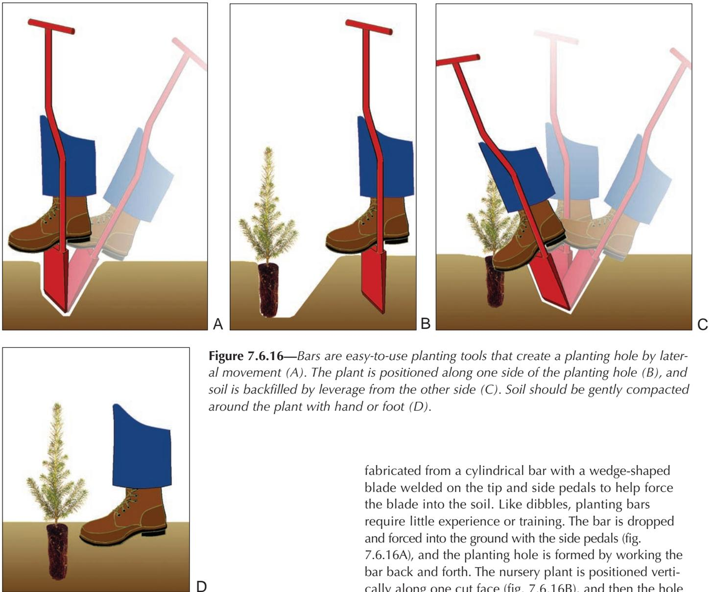
**Figure 7.6.16**—Bars are easy-to-use planting tools that create a planting hole by lateral movement (A). The plant is positioned along one side of the planting hole (B), and soil is backfilled by leverage from the other side (C). Soil should be gently compacted around the plant with hand or foot (D).
