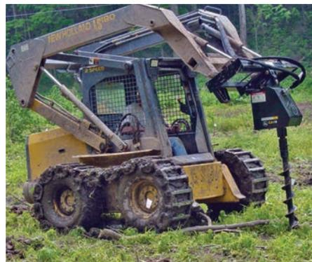
**Figure 7.6.20**—Augers are effective planting tools because one skilled operator can create planting holes (A&B) and several other workers plant the stock (C) and fill the holes by hand (D). Tractor-mounted augers can create holes large enough for the biggest container stock (E).
