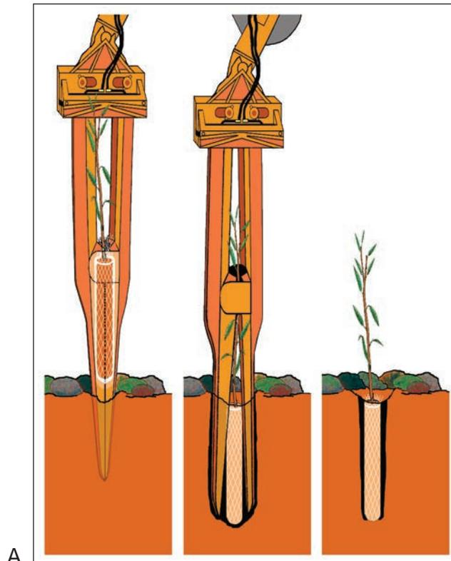
**Figure 7.6.23**—The expandable stinger is a specialized planting machine for harsh sites, including compacted soil and rip-rap (A). The long scissor-like planting head creates a planting hole where a tall pot container or nonrooted cutting can be installed (B).
