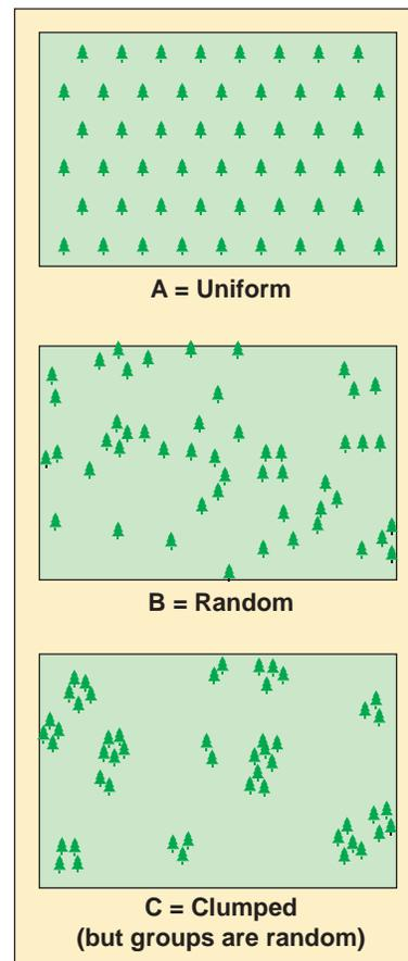
**Figure 7.6.11**—In addition to target plant specifications, the objectives of the outplanting project affect planting patterns. If the objective is rapid growth or Christmas trees, then plants can be regularly spaced (A). Most restoration projects do not want the “cornfield look,” however, so plants are spaced in a more random pattern to mimic natural conditions (B). The most natural outplanting look uses the random clumped pattern, where different species are planted in groups (C).
