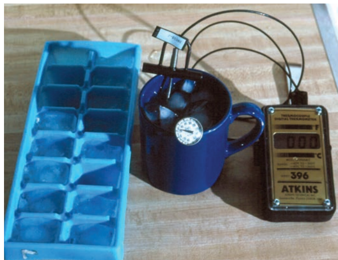
Figure 7.4.16 —Temperature can be monitored with long-stemmed electronic thermometers (A). Small hygrothermographs like the DataPod ® can monitor both temperature and relative humidity (B). Even smaller, the iButton ® can monitor temperature for weeks or months, and the data can be downloaded to a computer (C). Calibrate any thermometer in a water and ice mixture to make sure it is accurate (D).
