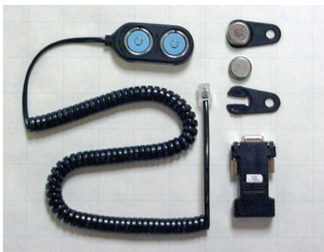
Figure 7.4.16 —Temperature can be monitored with long-stemmed electronic thermometers (A). Small hygrothermographs like the DataPod ® can monitor both temperature and relative humidity (B). Even smaller, the iButton ® can monitor temperature for weeks or months, and the data can be downloaded to a computer (C). Calibrate any thermometer in a water and ice mixture to make sure it is accurate (D).
