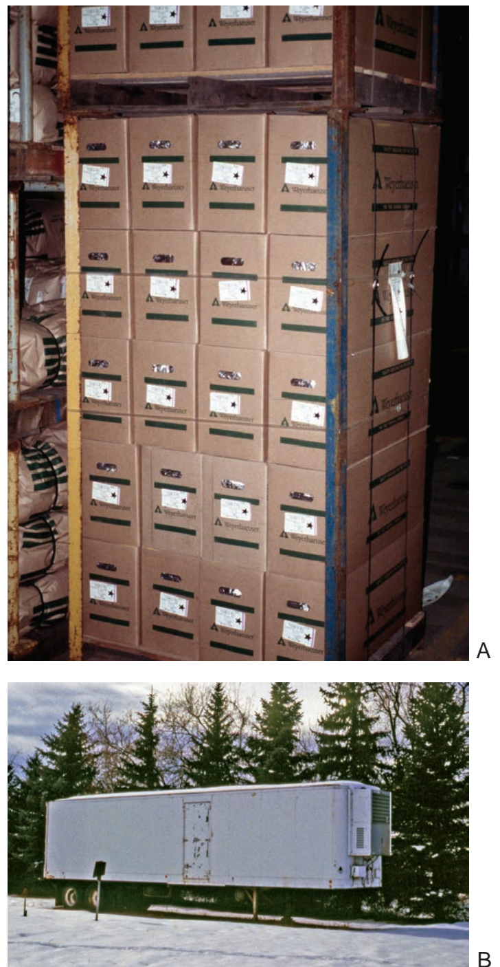
Figure 7.4.13 —To ensure uniform temperatures throughout the refrigerated storage units, boxes must be spaced on shelving to allow good air flow (A). Portable reefer vans (B) should be used only for short-term refrigerated storage.
