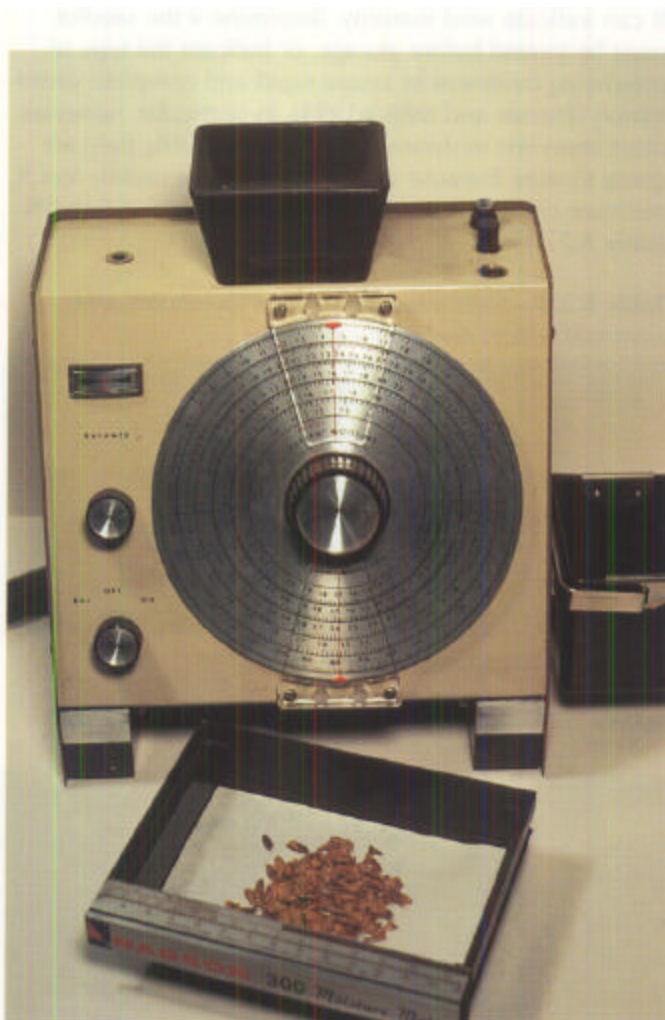
Figure 6.2.13 —Electronic moisture meters can give quick measurements of seed moisture content if they have been properly calibrated for the species (courtesy of R. Karrfalt, USDA Forest Service).
