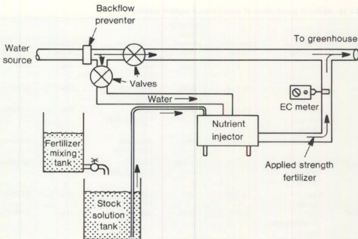
Figure 4.1.17—Schematic diagram of a typical liquid fertilizer injection system for a container nursery (adapted from Nelson 1978).
