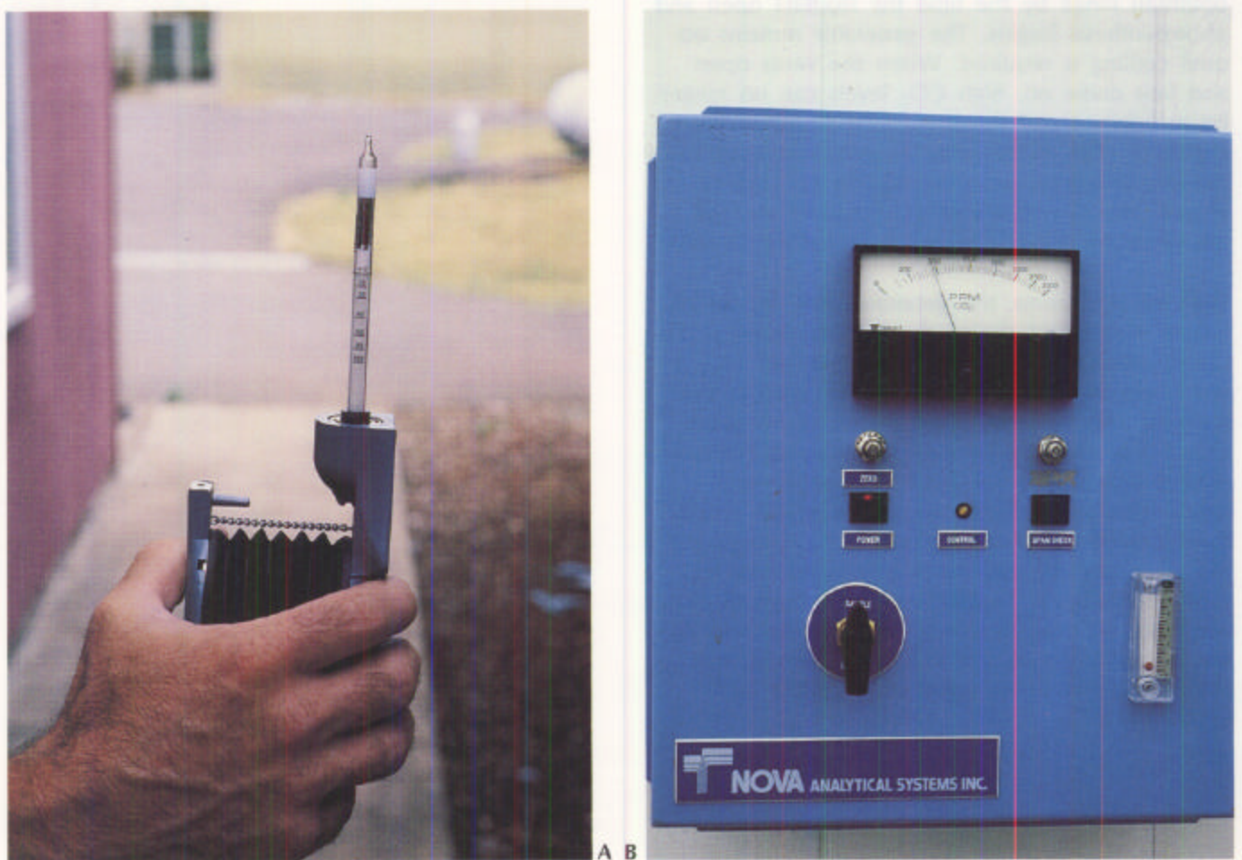
Figure 3.4.8 —Hand pump CO 2 testers (A) operate by forcing air through a glass tube that is filled with reactive chemicals. The CO 2 concentration is measured by the distance of the color change down the tube. More sophisticated and expensive infrared gas analyzers precisely monitor CO 2 levels and provide constant feedback to the generators (B).
