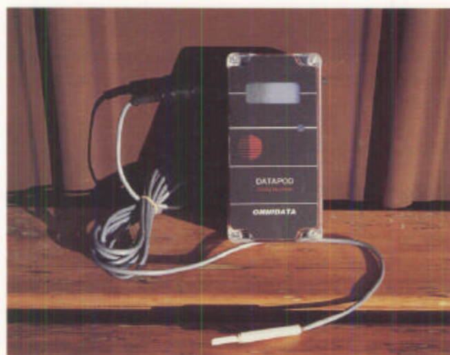
Figure 3.1.31 —Maximum-minimum (“max-min”) thermometers (A) measure current air temperature and also mark the high and low readings for a given time period. New electronic instruments have probes that are small enough to measure and record the temperature of the growing medium within the container (B). Hygrothermographs (C) have been traditionally used in container nurseries to record both air temperature and relative humidity.
