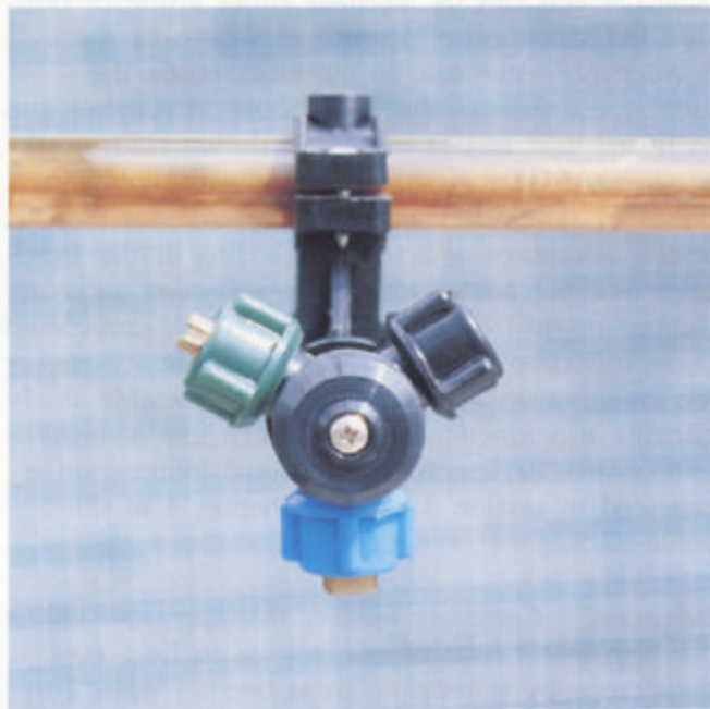
Figure 3.1.22 —Seedlings can be cooled by frequent, light irrigations. Some container nurseries have moveable irrigation booms (A) that are equipped with compound spray heads that contain a mist nozzle as well as the standard irrigation nozzle (B).
