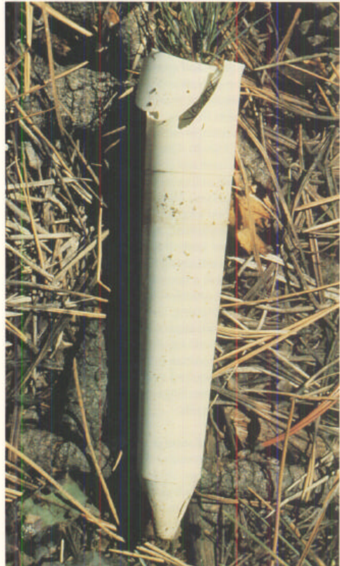
Figure 2.1.12 —Intense sunlight, especially ultraviolet radiation, can cause plastic containers to become brittle. Many containers are now constructed of plastics with “ultraviolet inhibiting” chemicals.
