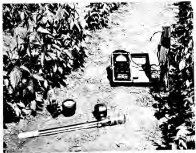
FIGURE 29.—Two instruments for soil moisture determination. The soil moisture meter on the left works on the tensiometer principle; it measures comparative soil dryness in terms of suction pull of the soil. The moisture meter on the right gages soil moisture electrometrically by measuring resistance of current through buried gypsum blocks.
