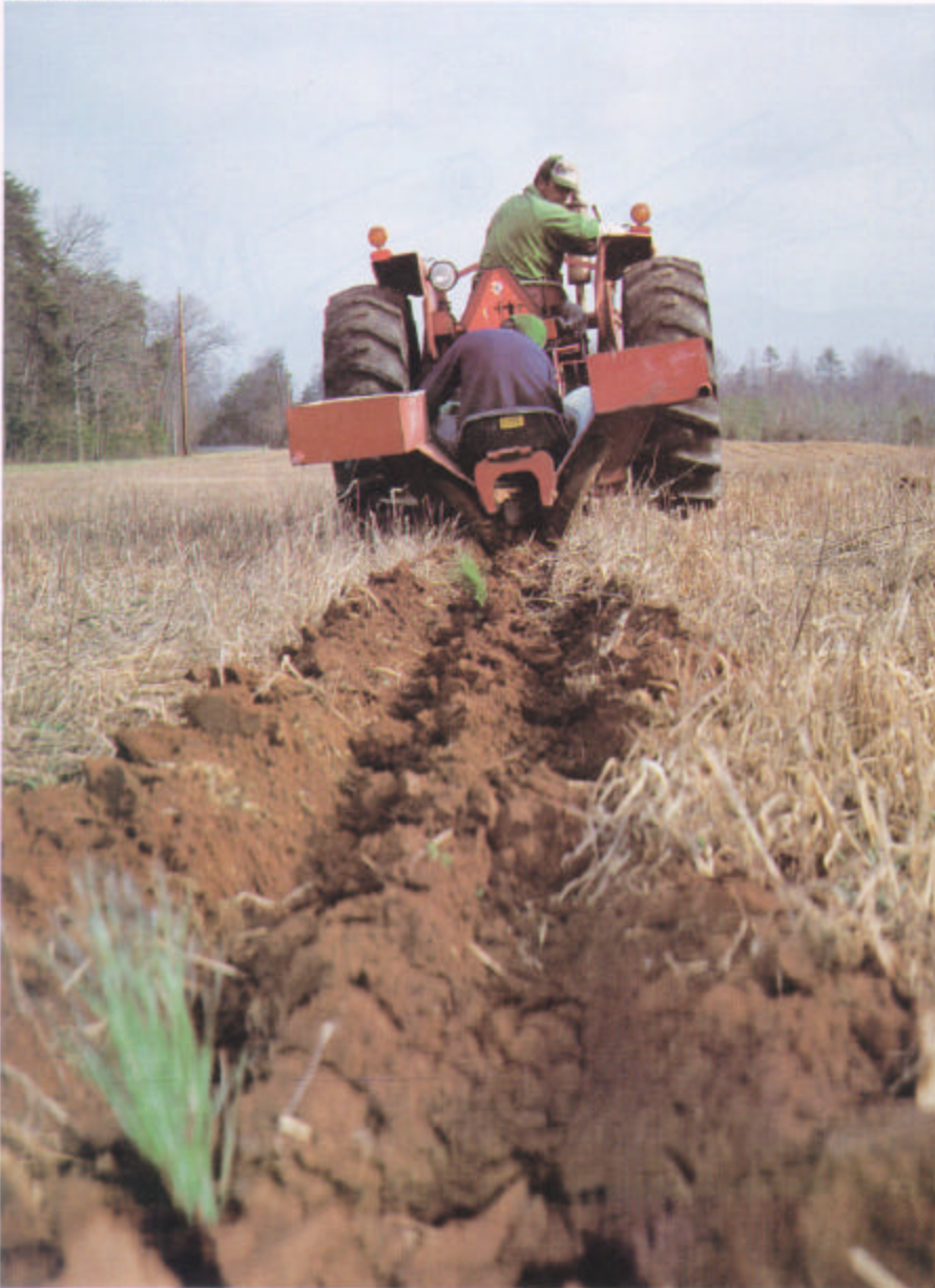
Careful machine planting places seedlings at the correct depth and spacing.
