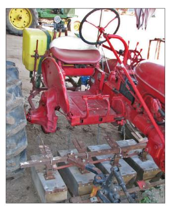
**Figure 8b.6**—This photograph shows an example of a shielded herbicide applicator designed for hardwood seedbeds. The advantage of this model is that it can be operated by one person. (Photo by David South, 2010.)
