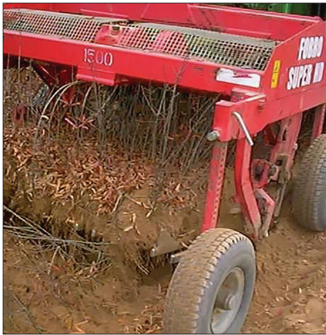
Figure 11c.1 —Fobro lifter showing the back tine tilt angle and height above bed. (Photo courtesy of Chase Weatherly, 2017.)
