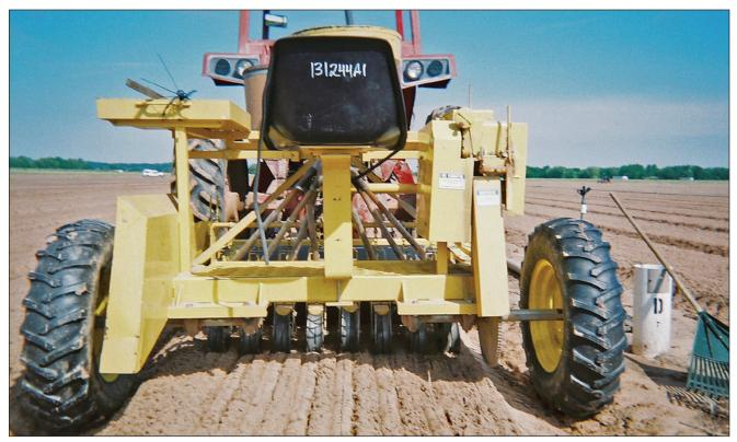
*Figure 4b.4*—A Love seeder showing drop tubes and rear packing wheels. The seeder accommodates up to eight drills and can be precision adjusted. (Photo courtesy of Louisiana Department of Agriculture and Forestry, 2005.)
