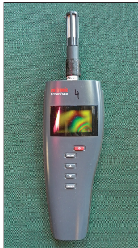
Figure 2.19—Handheld hygrometer for measuring equilibrium relative humidity of a seed lot. (Photo by R. Karrfalt, USDA Forest Service.)
