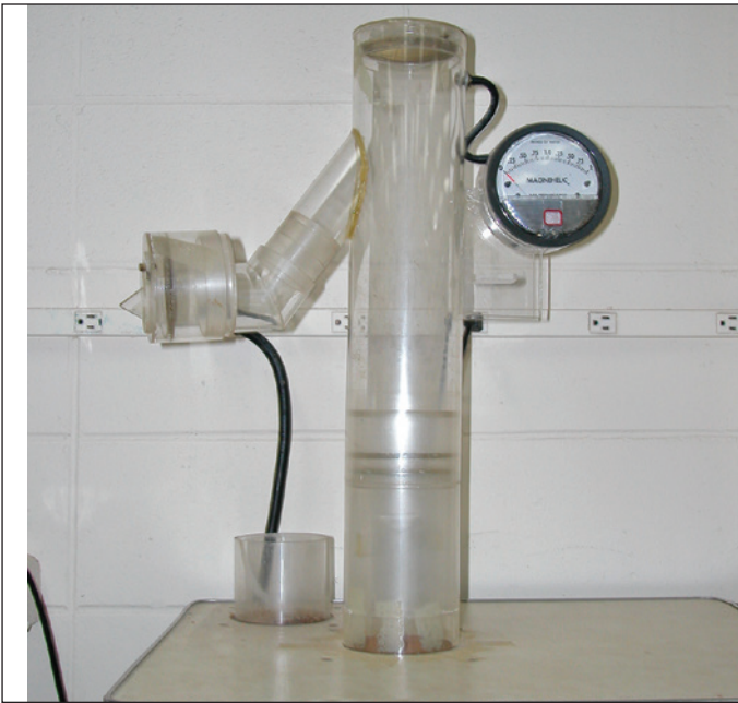
Figure 2.9 —This small blower removes trash with positive pressure. (Photo by R. Karrfalt, USDA Forest Service.)
