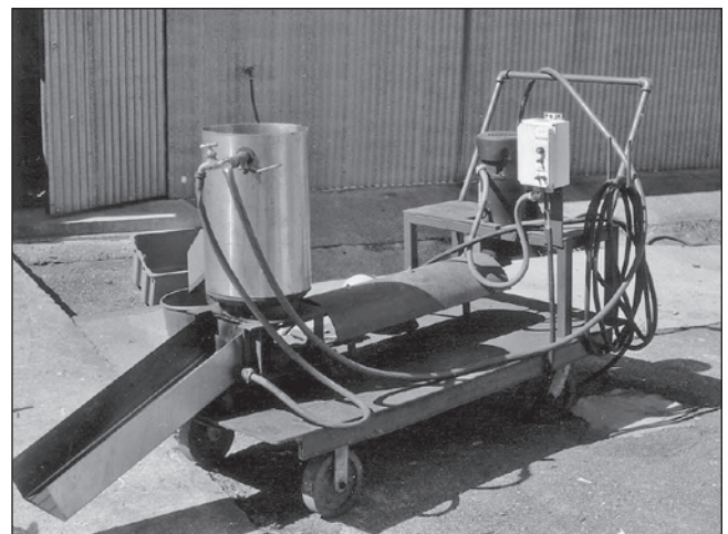
Figure 2.8 —A macerator for de-pulping fleshy fruited seeds. (Photo by R. Karrfalt, USDA Forest Service.)
