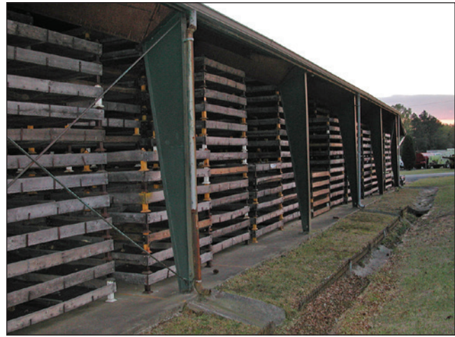
Figure 2.5 —Screen-bottomed racks for postharvest drying of seeds. Spacers allow natural air flow around each rack in the stack. (Photo by R. Karrfalt, USDA Forest Service.)
