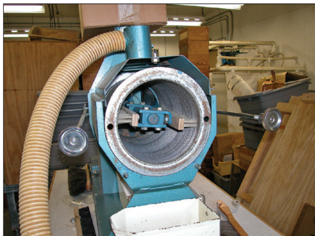
Figure 2.6 —Brush machine for hulling indehiscent fruits, dewinging and singularizing seeds. (Photo by R. Karrfalt, USDA Forest Service.)
