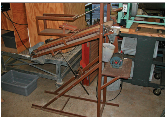
Figure 2.16 —The inclined draper separates particles on their ability to roll or slide down an inclined belt. (Photo by R. Karrfalt, USDA Forest Service.)
