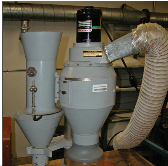
Figure 2.10 —A small aspirator removes trash with vacuum. (Photo by R. Karrfalt, USDA Forest Service.)
