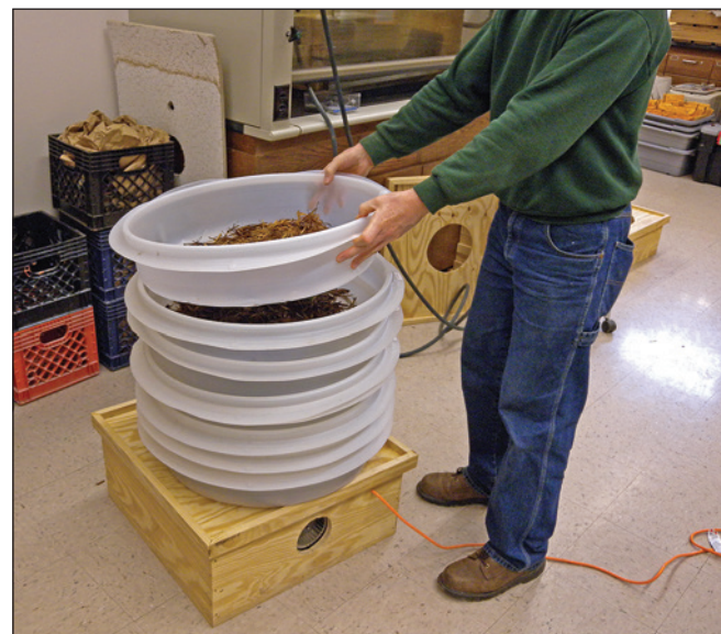
Figure 2.22 —A small pressurized seed drier. (Photo by R. Karrfalt, USDA Forest Service.)
