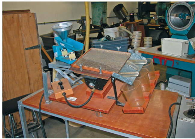
Figure 2.17 —The vibratory separator removes trash from seeds by differences in surface texture. (Photo by R. Karrfalt, USDA Forest Service.)
