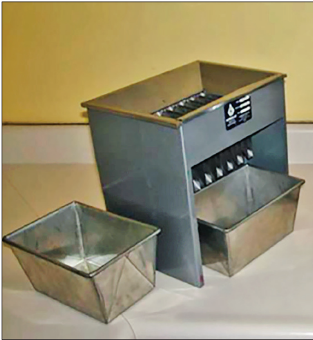
Figure 2.24 —Riffle divider. (Photo by R. Karrfalt, USDA Forest Service.)
