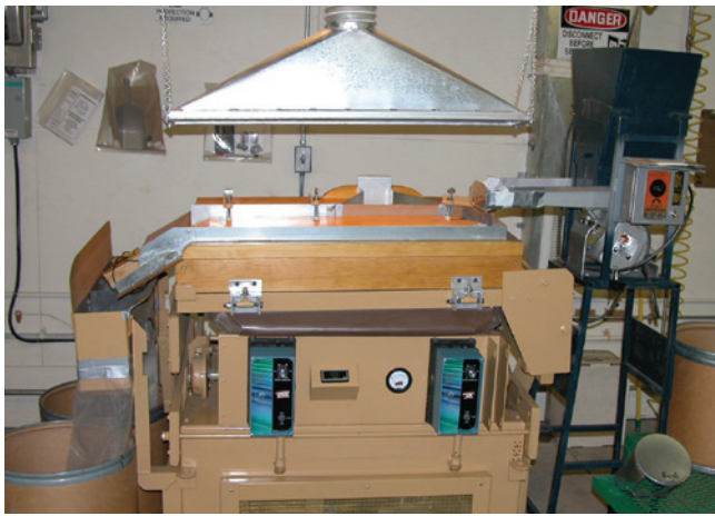
Figure 2.15 —A specific gravity table for separating seeds from trash using weight differences. (Photo by R. Karrfalt, USDA Forest Service.)
