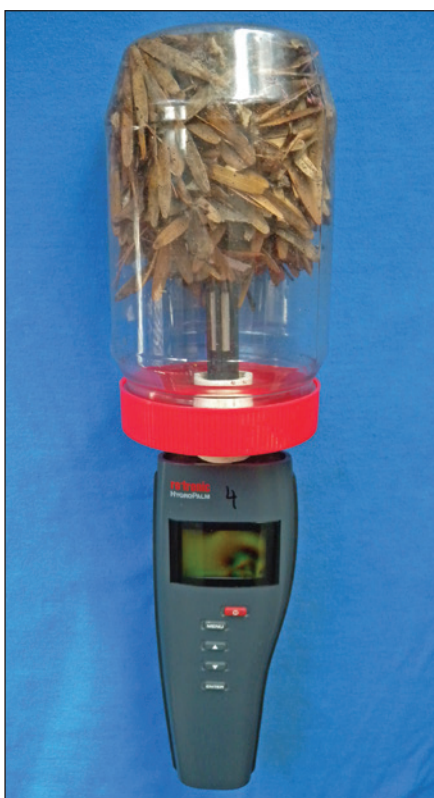
Figure 2.20 —A recycled peanut butter jar used as a test chamber for measuring equilibrium relative humidity (eRH) to test if the seed is dry for storage. A 30-percent eRH is good for all seeds that should be dried. (Photo by R. Karrfalt, USDA Forest Service.)
