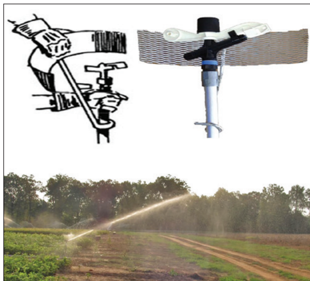
Figure 5.5 —Sprinkler shields can be used on full-circle sprinklers to prevent full-circle application. Some shields use solid splash plates and drop all the deflected water near the sprinkler, others use splash plates made of expanded metal to control overwatering near the sprinkler. (Photo courtesy of Irrigation-Mart and Chase Weatherly, ArborGen, Inc., 2011.)
