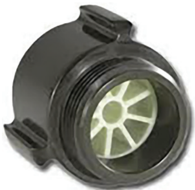
Figure 5.3 —Sprinkler nozzle with stream straightener vanes installed. A sprinkler's throw distance will be increased by 3 to 4 feet (.9 to 1.2 m) and the application uniformity will be greater if the streamlines exiting the sprinkler nozzles are straight. (Photo courtesy of Irrigation-Mart, 2011.)
