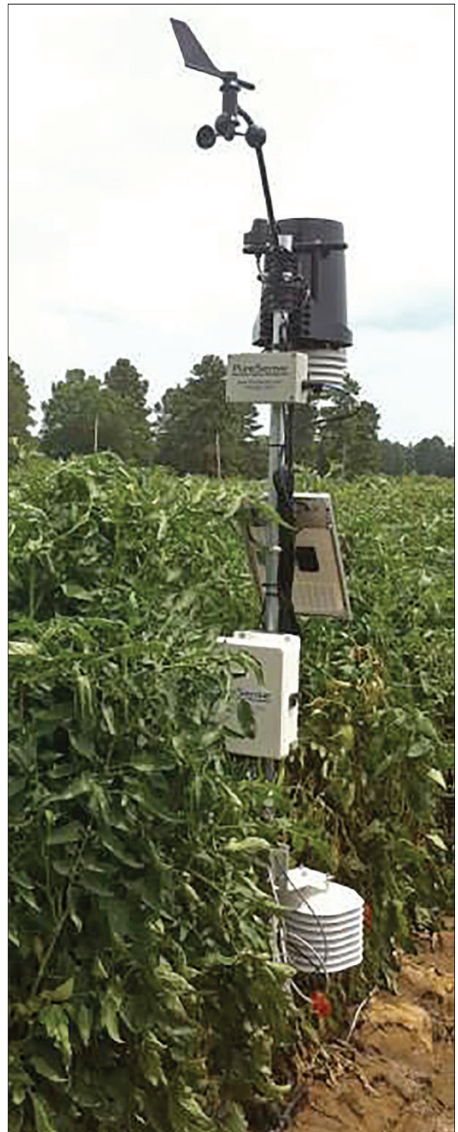
Figure 5.7 —Field station continuously measuring and transmitting volumetric soil moisture and salinity at various depths, in and out of canopy weather, and irrigation system pressure when irrigation is occurring. (Photo courtesy of Irrigation-Mart, 2011.)
