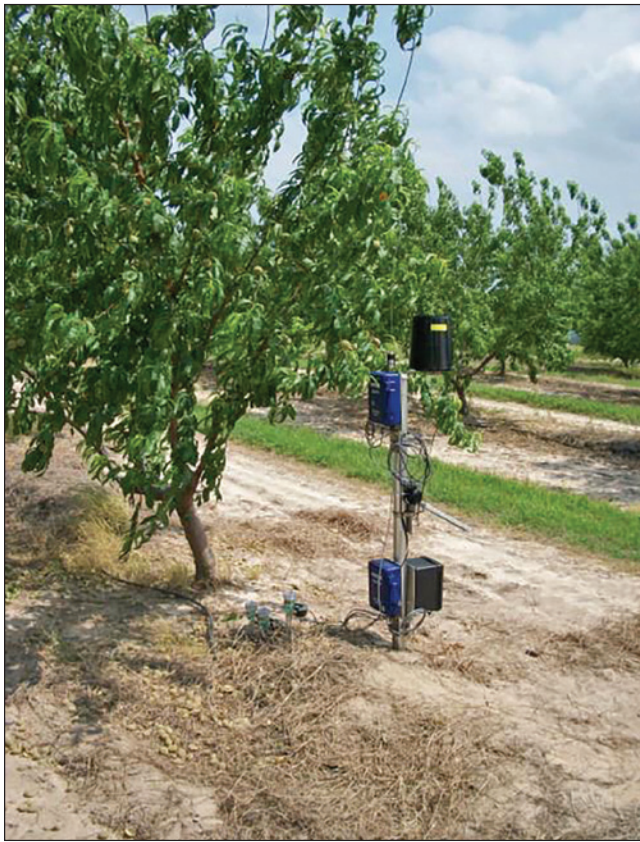
Figure 5.6 —Field station automatically measuring and transmitting tensiometric soil moisture and other soil indices at various depths. (Photo courtesy of Irrigation-Mart, 2011.)
