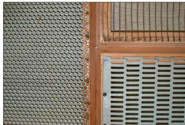
**Figure 2.11**—Hand screens showing the three main types of screens used to clean seedlots (counter-clockwise from left): perforated metal round hole, perforated metal oblong holes, and woven wire. (Photo by R. Karrfalt, USDA Forest Service.)
