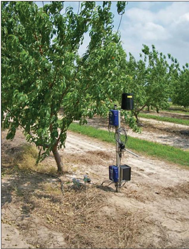
**Figure 5.6**—Field station automatically measuring and transmitting tensiometric soil moisture and other soil indices at various depths. (Photo courtesy of Irrigation-Mart, 2011.)
