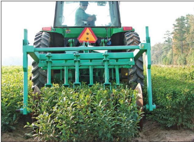
**Figure 11d.8**—Whitfield® lateral pruner over sawtooth oak. (Photo by R. Cross.)
