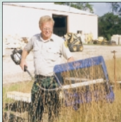
Figure 3 • Prairie seed stripper used for seed collection on wiregrass sites.
