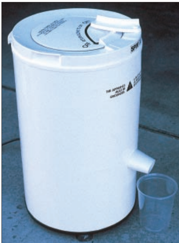
Figure 1 • A laundry spin dryer can be used to remove surface water from seeds.
